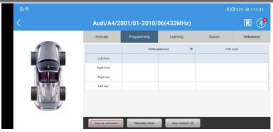
2) If the tip shown as below pops up, you need to activate the original sensor first. Click the **【Ok】** to transfer to the **Activate** interface.
