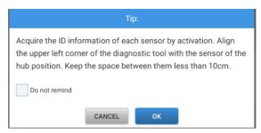
Keep the tool top close to the sensor from the outer edge of the tire. If failed, try to do it from different tire position or direction.
